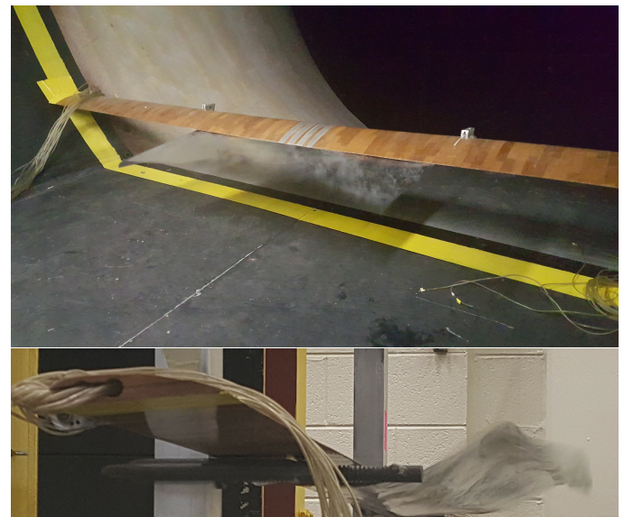
Figure 5. 5: Wind tunnel tests of the Flying Carpet. Top: High aspect ratio sheet attached to the bottom of a flying wing, remaining steady at low wind speed. Bottom: Sheet exhibiting periodic flag flutter instability.
